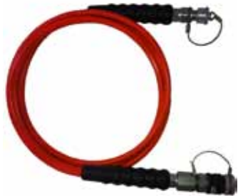
Model No. 170205 "HOSE" 5m (Orange) 850bar Working Pressure Non Conductive with Cejn M&F 10-116 series Couplings & Aluminium dust caps
