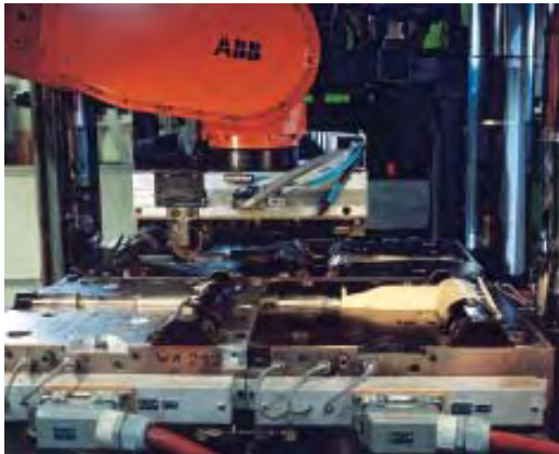
Manufacturing of premoulded connectors takes place in accordance with a unique method, in which different layers are vulcanized together.
