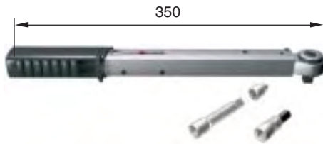
730 R Torque wrench for screw connectors, screw cable lugs, overhead line clamps, etc. Supplied with 7 mm socket head, extension and 8 mm internal hexagon head. Torque range 6-50 Nm.
