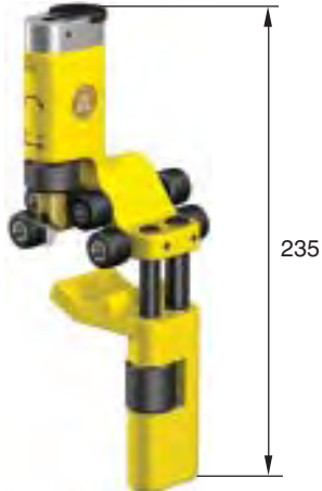
GB-M20 Cutting tool for cable sheath and XLPE insulation: Diameter: \varnothing 15-50 mm Cutting depth: \leq 8 mm
