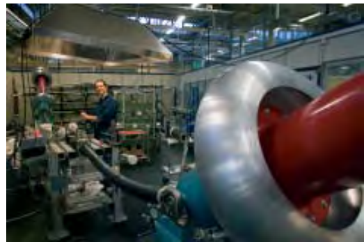
Routine testing of high voltage cable joints.
