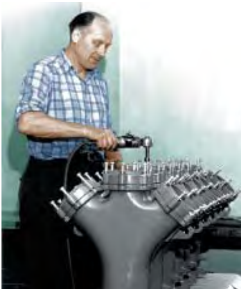
Manufacturing outdoor cable terminations for paper-insulated cables in 1962.
