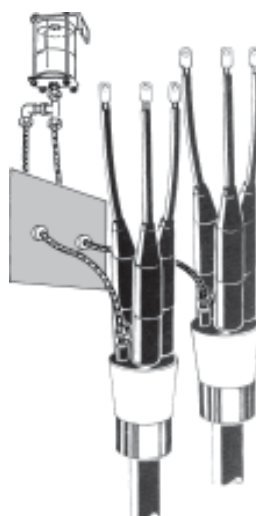
GEX 02 Expansion vessel for two OTIA 152.
