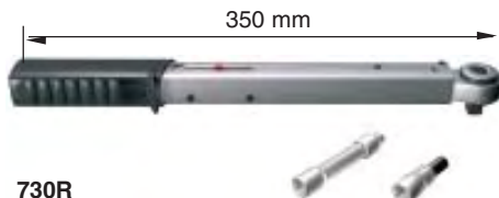
730R Torque wrench for screw connectors, screw cable lugs, overhead line clamps, etc. Supplied with 7 mm socket head, extension arm and 8 mm internal hexagon head. Torque range 6-50 Nm.
