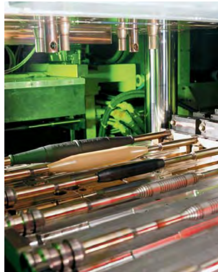
The three layers of the joint are vulcanized together in a unique manufacturing process.
