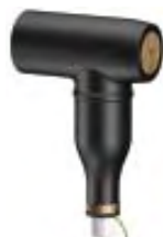
IH SOC 630 Sealing hood of HD-polyethylene, to be installed in SOC instead of cable in order to temporarily insulate 630 A switchgear or transformer bushings.
