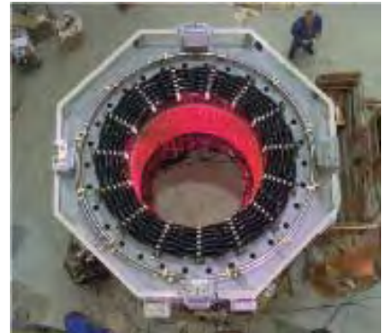
SOJ is used for jointing of the winding in a Powerformer, Sweden.
