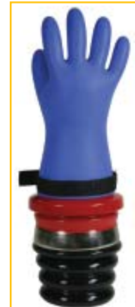
G100 with inflated lo-volt glove ready for inspection.
