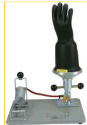
G2 with inflated glove ready for inspection.
