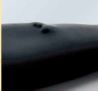
Chemical Attack: This photo shows swelling caused by oils and petroleum compounds.
