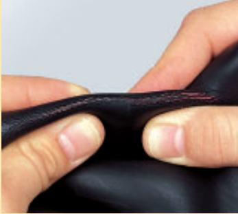
Cracking & Cutting: This type of damage is caused by prolonged folding or compressing.
