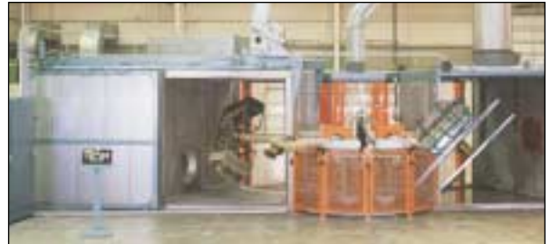
Typical multi arm carousel rotational moulding machine, showing oven, cooling chamber and loading / unloading area.
